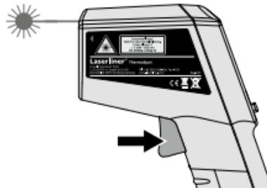
Release the button as soon as the laser circle pinpoints the measurement location. The measured value is held.
