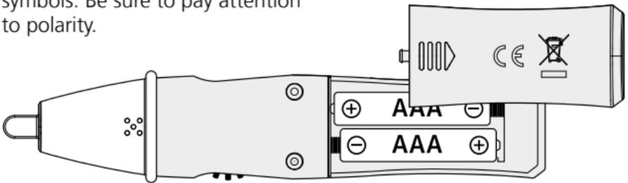
**!** Before using the device, you should always test it on a main circuit you know to be operational within the specified voltage range. To avoid inaccurate measurements, check the device batteries prior to use by switching on the built-in battery lamp (see 5).
